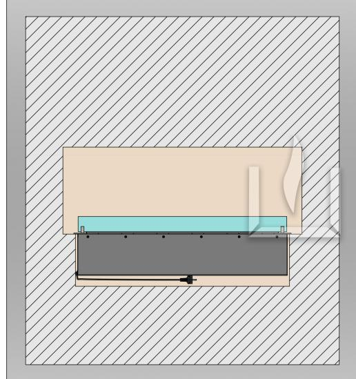
Installing a fireplace in a solid wall. Recommended installation option.
