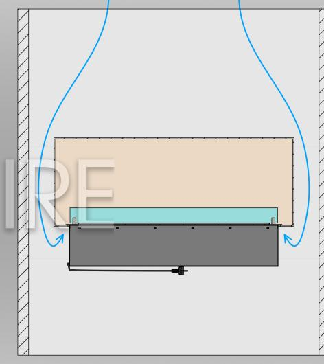
Installing a fireplace in a hollow wall design, which is open above and below the niche for the hearth (without additional partitions). Warm the air inside the wall will cause negative flows that negatively will affect the line of fire. Forbidden installation option.
