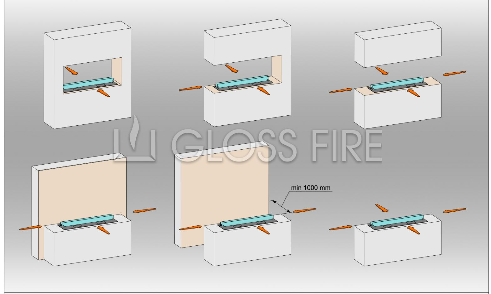
Attention! Installing glass on a biofireplace is mandatory. Do not operate the biofireplace without a vertically installed glass. Provide a Euro-type plug socket next to the bio-fireplace.
